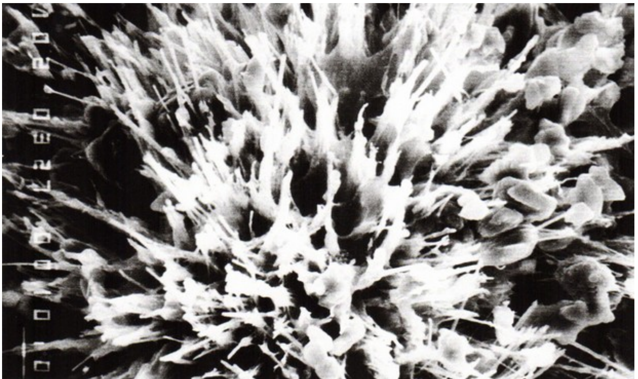
Dengta Xypex Concentrate, 50mm gylyje
